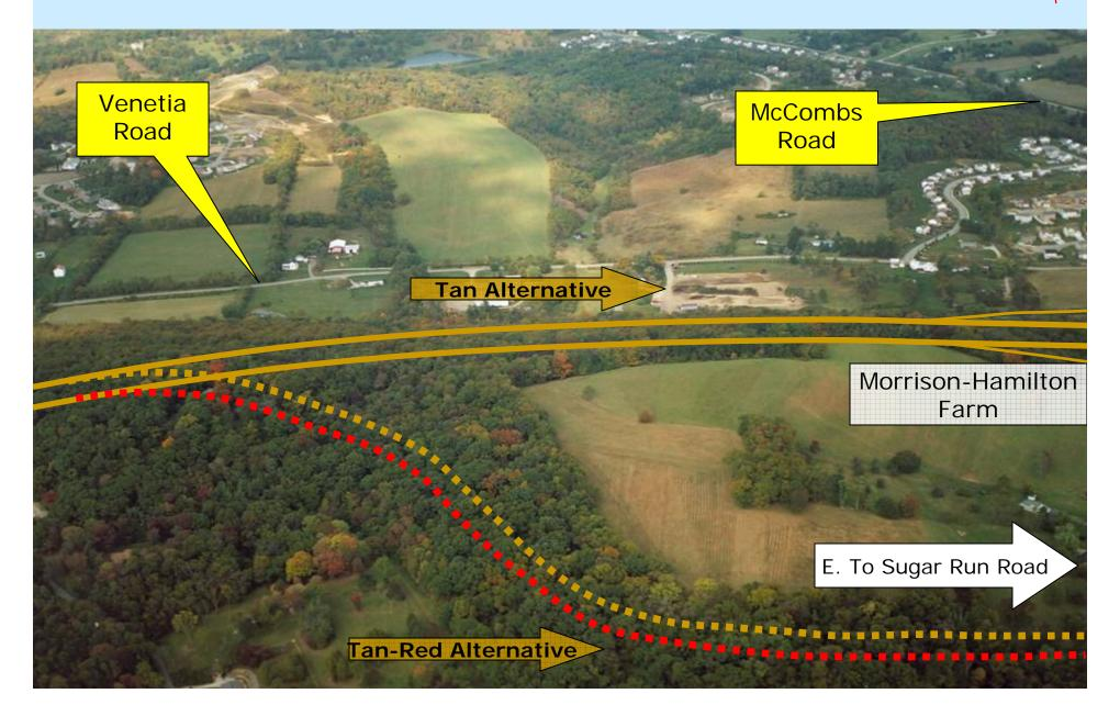
I-79 to Mon/Fayette Expressway – Tan Alternative – Section 2 The Tan Alternative would interchange with Sugar Run Road in Nottingham Township. Sugar Run Road would be relocated to meet with Bebout Road, and a portion of Lutes Road would be relocated.
